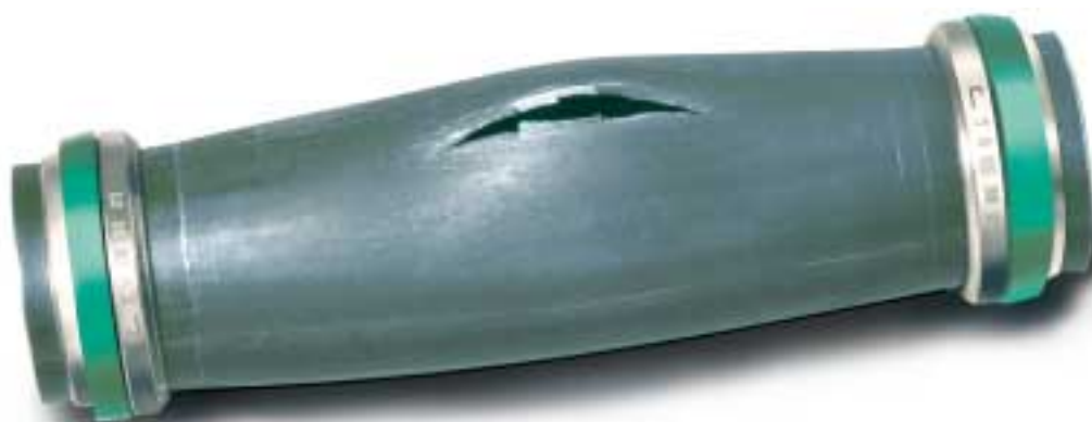
Destructive testing with 28x2 carbon steel tube The tube burst at 650 bar without any leakages or sweating from the sealing points
